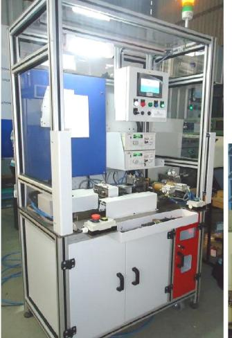
**Application** : EOT – Leak and Performance testing for Brake system pump
