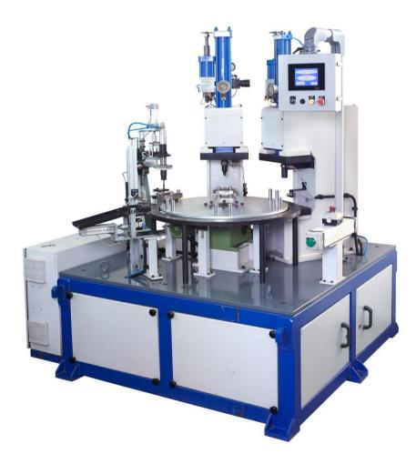
Application – Nut & Bracket Assembly Design Elements : Press structure, Pressing dolly, component fixture, etc, Retaping head & auto – unloading system Component - Nut & Bracket Cycle Time – 6 sec/component Pressing Force – 4 Ton
