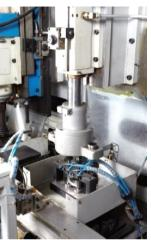
Application – Conventional Auto Drilling, Milling, Reaming Machine Design Elements : Support L – Structure, Walking beam with servo slide, Pick and Place for the component, programming
