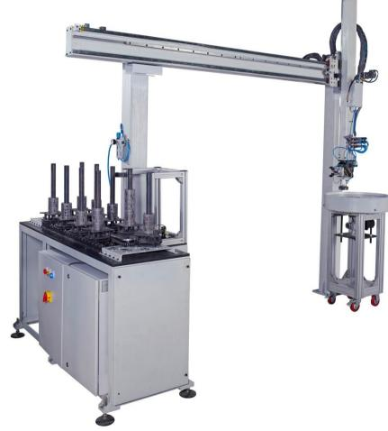
Application : Loading and Unloading system of synchro hub from stacker to CNC Machine Loading Indexer : 9 stations linear indexer with stack bars Gantry : X-axis and Z-axis Servo Driven Unloading Rotary Feeder : Driven by Motor and Gearbox
