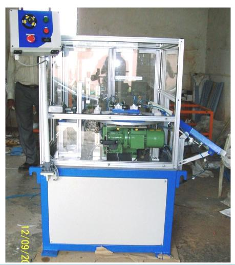
Application:- Refrigerator door switches continuity testing & ok-not ok marking.
