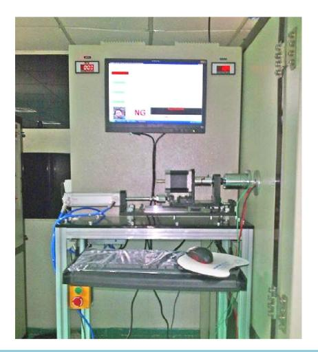
**Application:-**Ignition Switch endurance testing in environmental chamber.
