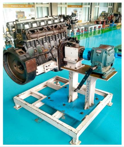
Application:-Engine rotation Design Elements:- Base frame, manual gearbox, spindle housing, indexing fixture to accommodate 4 variants
