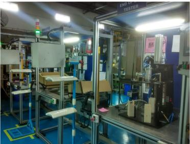
Application – Steering wheel & switch assembly & switch testing Design Elements : Al. station frame, St. wheel tilt fixture, DC screw driver, EOL switch testing, barcode printing
