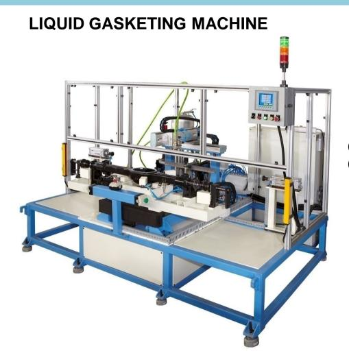
**Application** : Robotic RTV Application and Oil Seal pressing
